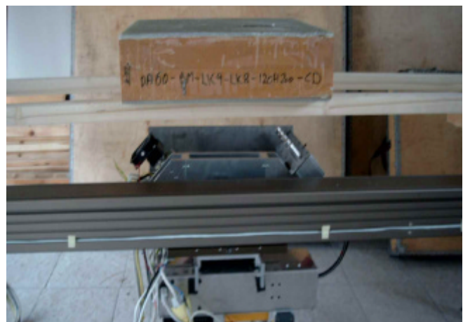
Fig. 1 (left) and 2. The backscatter assembly mounted in a cabinet (object moving) or on a linear guide with stationary object (right).
