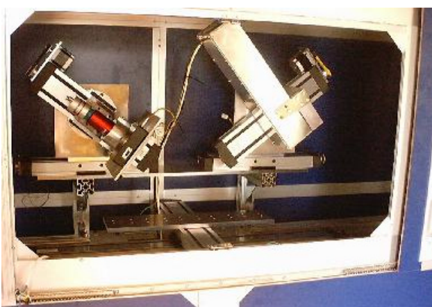
Fig. 1 (left) and 2. The backscatter assembly mounted in a cabinet (object moving) or on a linear guide with stationary object (right).
