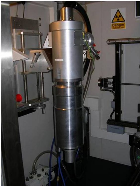
Figure 1 Prototype 450kV microfocus X-Ray source.
