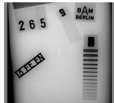
Radiograph of sample showing induced thermal fatigue crack
